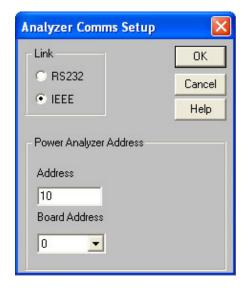
Alternatively, if you are using a serial interface, click with the mouse on the RS232 button, enter the appropriate Comm Port and Baud Rate, and then click the OK button.
