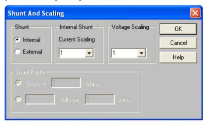
If the transformer is not 1:1, you should enter the appropriate current (or voltage) scaling factor before clicking on OK.
