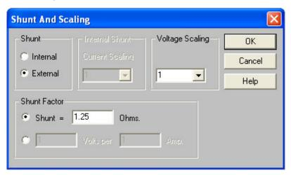
and enter the value of the shunt in the Shunt Factor section at the bottom of the dialogue box. Note that you may enter either an Ohmic value by selecting the upper button as shown in the display above, or a Volts per Amp ratio by clicking on the lower button.
