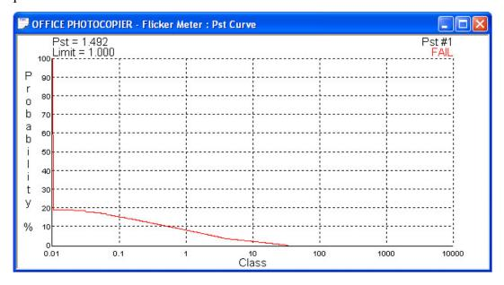
There will be a series of Pst curves - one for each ten-minute period in the measurement. You may view each curve in turn by using the < (less than) and > (greater than) keys to scroll through the series.
