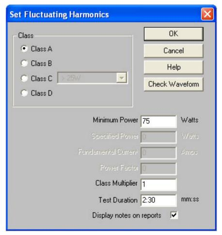
Select the Class (A, B, C or D) that the equipment belongs to. (See Chapter 2.) The correct limits will automatically be chosen. The other possible entries into this dialogue are described below.
