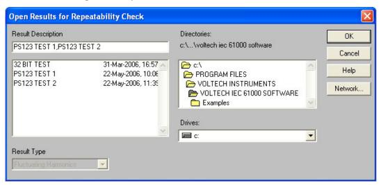
The repeatability test compares all the harmonic results for each harmonic from one set of results to every other to see if they are within 5%. Harmonics less than 0.6% of the input current or less than 5mA are ignored.
