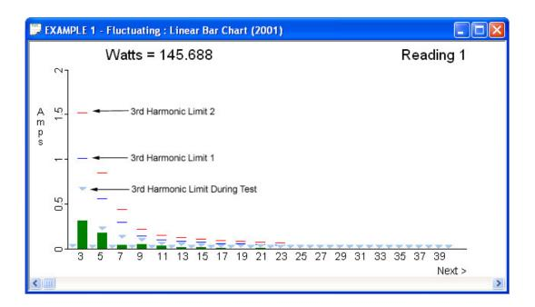
Use the play and pause keys to scan through each reading automatically or use the < (less than) and > (greater than) keys of the keyboard to scan through the readings one at a time.
