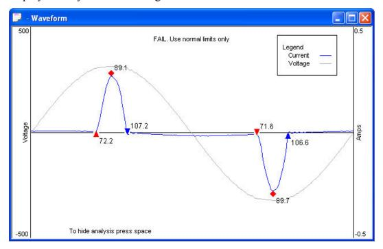
This waveform can then be used to check if Class C 'by waveform' limits can be used by pressing the space bar. The markers show the angular position of current 'flow start', 'last peak' and 'flow stop'.
