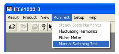
During the test the software automatically displays an ON prompt soon after the beginning of a one-minute test period and an OFF prompt before the end of a one-minute period.
