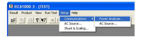
If you are using an IEEE488 interface, then enter the address of the Power Analyzer, and click on the OK button.
