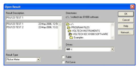
Initially change to the appropriate Drive and Directory. Then select the Result Type from the list revealed by clicking on the ▼ button; this will bring up a list of available results in the Result Description box. Finally, select the required result from the list by double-clicking with the mouse. This will close the dialogue box, and add the selected result to those already on view.
