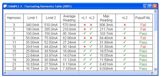
In the example above, the results for harmonic 5 show that the average result has exceeded limit 1 but not limit 2 and that the maximum reading has not exceeded limit 2 resulting in a FAIL for harmonic 5. See the reference information for more details.
