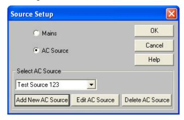
you can choose to have the software automatically control an AC Source or to use the normal line supply ('Mains') / manually controlled source.
