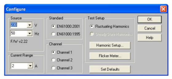
Again using the mouse to move between the various fields, set up the following:
