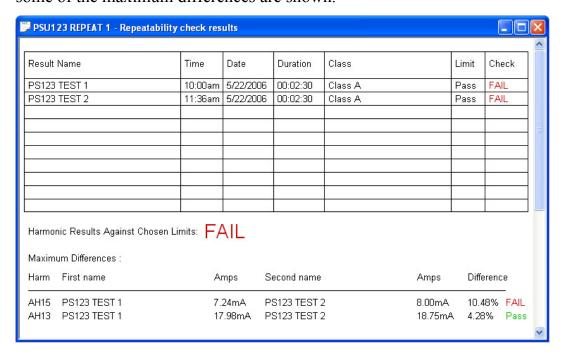
Should the repeatability test fail, ensure that the results selected refer to the same product tested under identical conditions.
