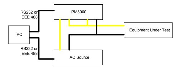
In many cases, you will be able to use a single test rig for the evaluation of a number of different products to the IEC61000-3 specification. Therefore, the IEC61000-3 software has a 'Setup' menu, which allows you to configure the test equipment and the type of test to perform first.
