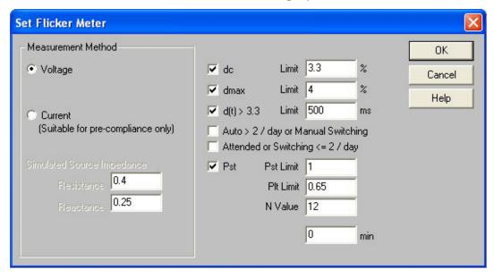
Normally, for full compliance testing, you would set the Measurement Method to Voltage, which would require you to insert a standard impedance network in the power line to the product under test. However, assuming that this time you want to use the measurement rig shown above for pre-compliance testing, click on the Current button in the Measurement Method box; the Resistance and Reactance default to the normal values specified in the IEC61000-3-3 Standard.
