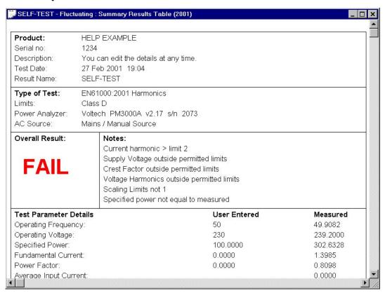
This is a summary test report showing the overall test PASS / FAIL together with all the product and test details.
