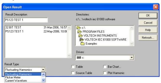
Select the 'Result Type' ('Fluctuating Harmonics' in this example), locate the result you wish to open and double click on it.
