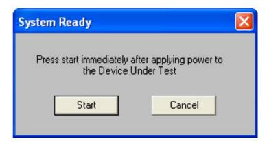
As for the Fluctuating Harmonics test, ensure that the Mains supply is connected to the Product Under Test at the first display and click on the OK button. At the second display, ensure that the Product Under Test is switched on and has settled into steady state operation, and then click on the Start button.
