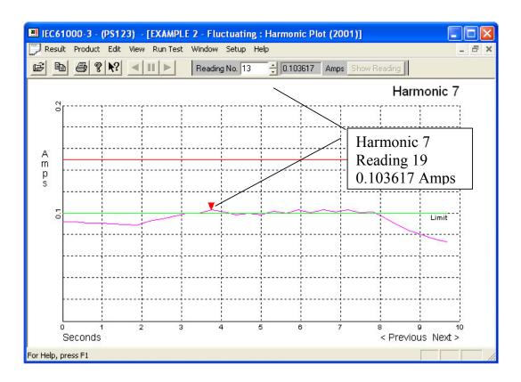
Use the < (less than) and > (greater than) keyboard keys to view the different harmonics.
